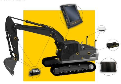
Components: Tilt sensor (optional), Bucket sensor, Boom sensor, Arm Sensor, Frame sensor, Display unit (8,4"), GNSS masts (or Rail mounts), GNSS antennas, GNSS receiver, Control unit
